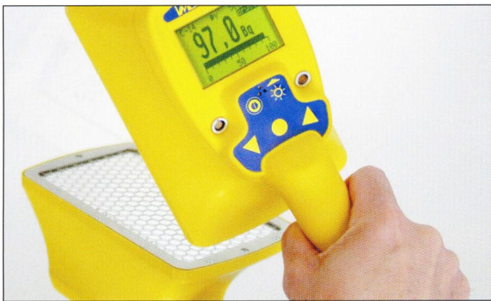
*Monitor with plastic scintillator for radioactive contamination measurement of surfaces in nuclear medicine laboratories*
