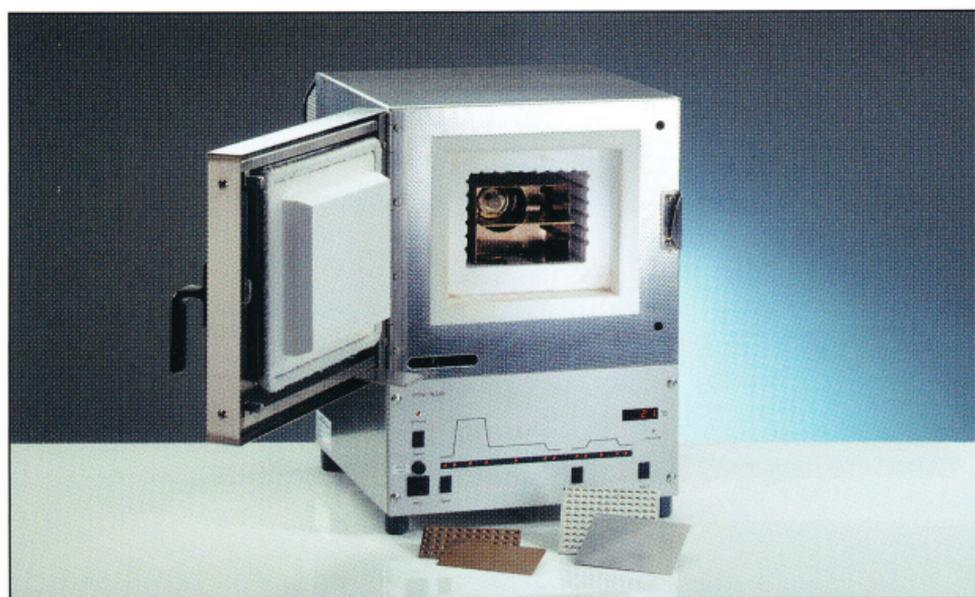
*Preheating and annealing oven with two standard programs; Programmable via an RS232 interface with THELDO software*
