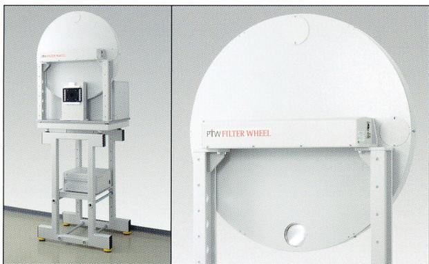
*Basic construction to accommodate an X-ray tube, X-RAY SHUTTER, FILTER WHEEL and filters*
