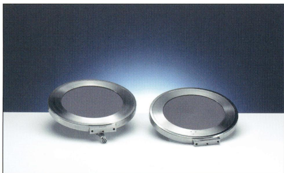
*Large size plane parallel transmission chambers for use as dose monitors combined with calibration facilities*
