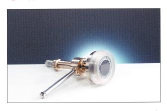
Low energy extrapolation chamber with adjustable volume depth for measure-ment of absorbed dose in soft tissue
