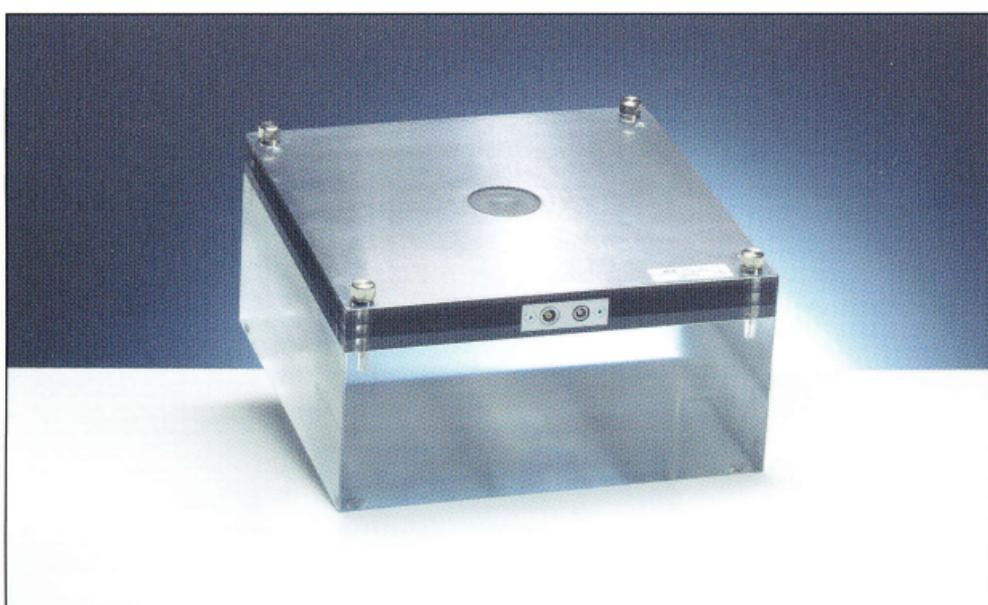
*Parallel plate ionization chamber for direct measurement of  $H_p(10)$  personal dose equivalent on a slab phantom*
