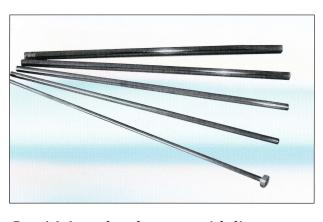
Sensitivity tube phantom with line source tube for quality control of positron emission tomographs (PET scanners)
