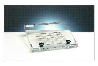
Test device for checking the dwell positions of afterloading sources
